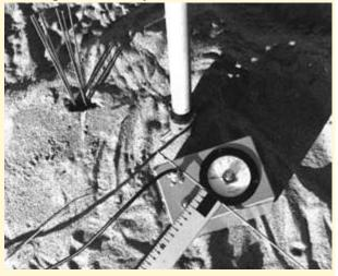
Once the experimenter has confidence in the integrity of the antenna range, it's quite possible to dispense with the receiver and VU meter and use a signal source plus a field strength meter such as the one shown in the photo at right (which also shows an
