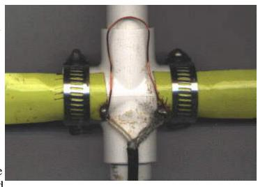
that the SWR was 1:1 at 146.565 Mhz (our Fox-Hunt frequency) when the two elements were spaced approximately 1 inch apart. Figure 1 shows the method used to attach the driven element to the PVC cross.
