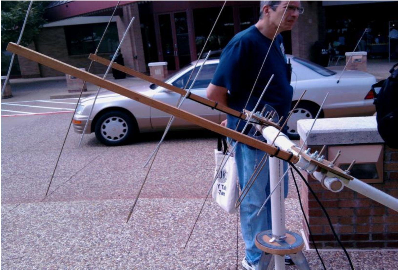
2011 - 2 Meter LFA (G0KSC) & 10 element 440 Yagi Azimuth Rotor
