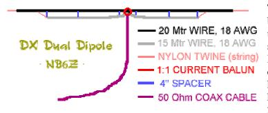
The antenna diagram you see before you is nothing more than two dipoles fed from the same coaxial line. I call it a " DX Dual Dipole" because it is cut for two very useful DXing ham bands. There is no harmonic relationship between 20 and 15 meters, and so they
